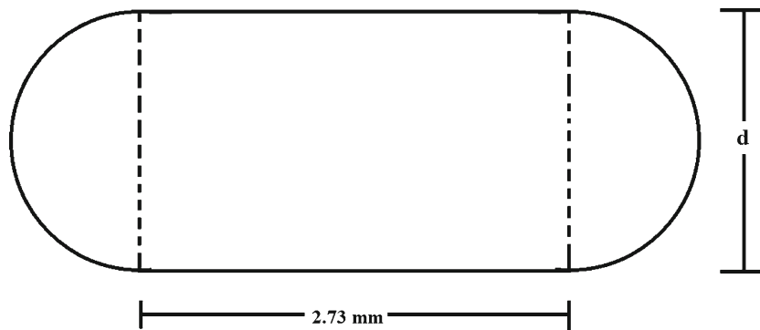
Fig. 4. Schematic diagram of shape of scanned area by NIR probe ( d diameter of probe) in dynamic mode
